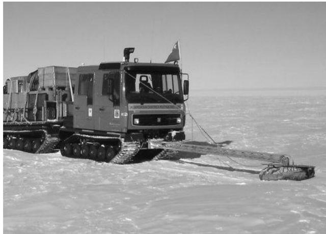
**Fig. 5** Ground penetrating radar mounted on a 7-m long metal rod in front of the BERCO TL6 tractor, East Antarctica. The radar transducer is installed inside the rubber inner tube at the right end of the rod, which is connected with a cable to the digital control unit installed in the tractor cabin.
