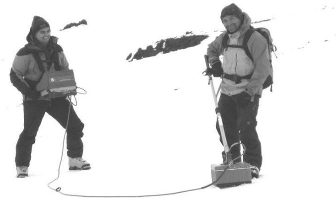
**Fig. 4** Ground Penetrating Radar used on Volcán Mocho-Choshuenco, Chilean Lake District. The operator on the left has the digital control unit, while the person on the right carries the transducer.
