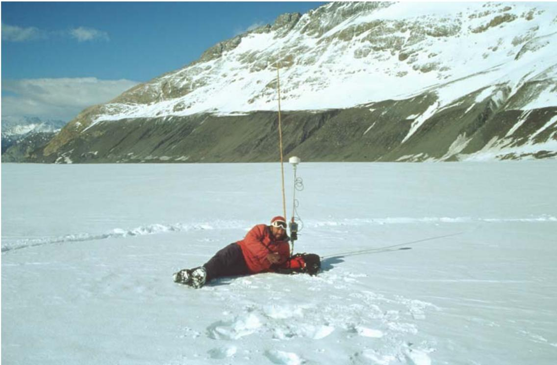
*Figure 2.3 The author of this thesis measuring in September 2001 one of the stakes installed on Glaciar Chico near the ELA of the glacier, using a geodetic quality GPS receiver.*
