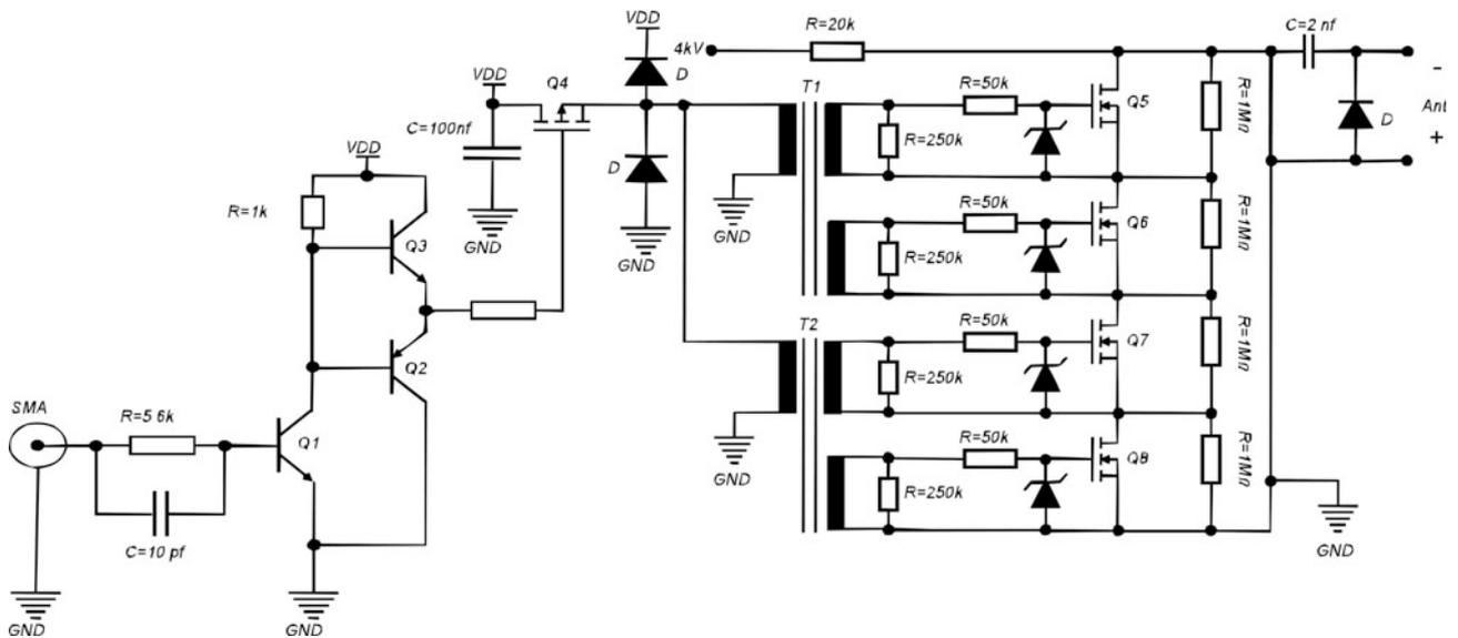
**Fig. 3.** Transmitter power circuit schematic of negative pulser. Upper left ports are used for the high-voltage power supply, lower left ports command the impulse instant and right ports correspond to the pulser output (complementary to the positive modulator).
