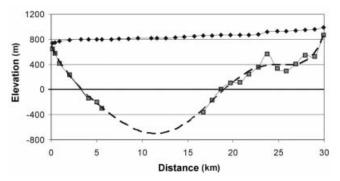
**Fig. 9.** Cross-section of Horseshoe Valley, from the margin of the BIA at Patriot Hills (station P1 on the left of the graph) to a point 30 km north (H34 on the right of the graph), at the foot of Douglas Peaks. Diamonds correspond to the surface elevation of stakes, measured by GPS. Squares are bed elevations measured with ice radar. The dashed line is a polynomial interpolation of the radar data. The maximum interpolated ice thickness is 1520 m.
